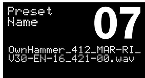
To exit just make a single short press on the **ENCODER (7)** and you'll find yourself in the main display's screen (the main mode of the presets switching).
