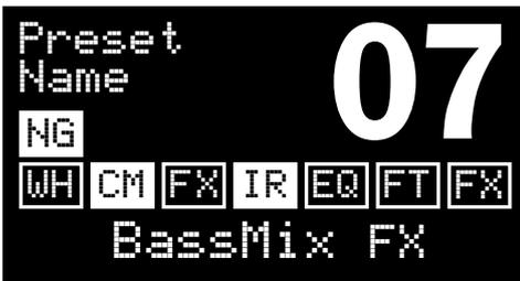
To enter into the viewing screen with the name of WAV IR (Impulse Response) of the Preset, make a single short press on the **ENCODER (7)**.
