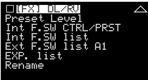
To enter inside of any menu item, just go to the necessary menu string on the Ultima's display and push the **ENCODER (7)**. For example, if we will enter inside of the menu item **[FX] DL/RV**, we'll see another submenu with its own settings:
