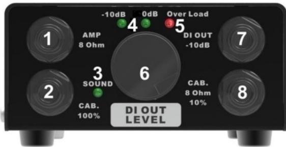
1. “AMP 8 Ohm” – Jack Socket for Power amp output (load 8 Ohm).
