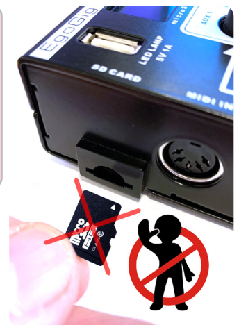
Fig. 1. — An example of the correct (left - «contacts up») and incorrect (right — «contacts down») orientation of the microSD memory card in space relative to the AMT Agogic EG-4 device
