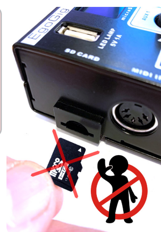
Fig. 1. — An example of the correct (left - «contacts up») and incorrect (right — «contacts down») orientation of the microSD memory card in space relative to the AMT Agogic EG-4 device
