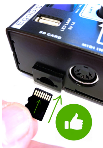
Fig. 1. — An example of the correct (left - «contacts up») and incorrect (right — «contacts down») orientation of the microSD memory card in space relative to the AMT Agogic EG-4 device
