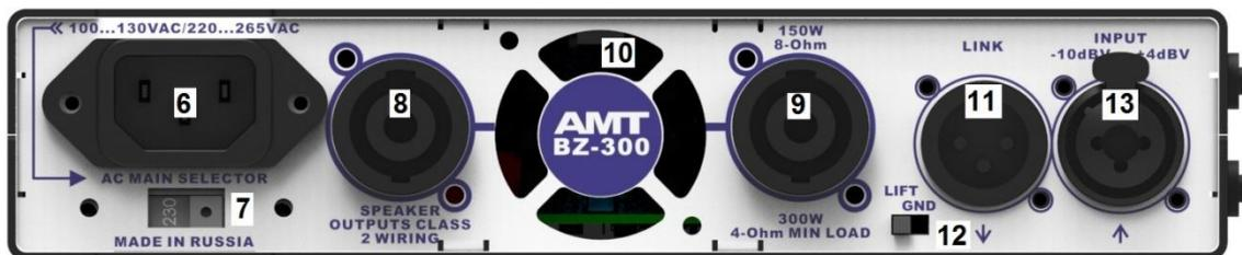
6. **AC mains power socket.** This is where you connect the supplied AC power cord.
