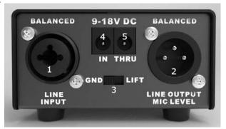
1. LINE INPUT (balanced or unbalanced line input) – combined XLR/TRS socket. You can plug in it a cable from your Sound Card (DAW) output. It can be an XLR – XLR balanced cable, a TRS-TRS balanced cable or a TS-TS unbalanced cable.
